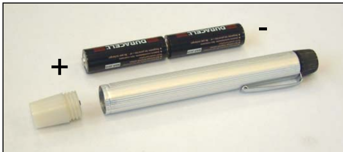
Figure 1. Microscope light source - battery polarity
