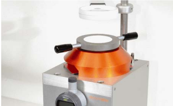
Figure 3. Metal sheet clamped in the die and ready for cupping test
